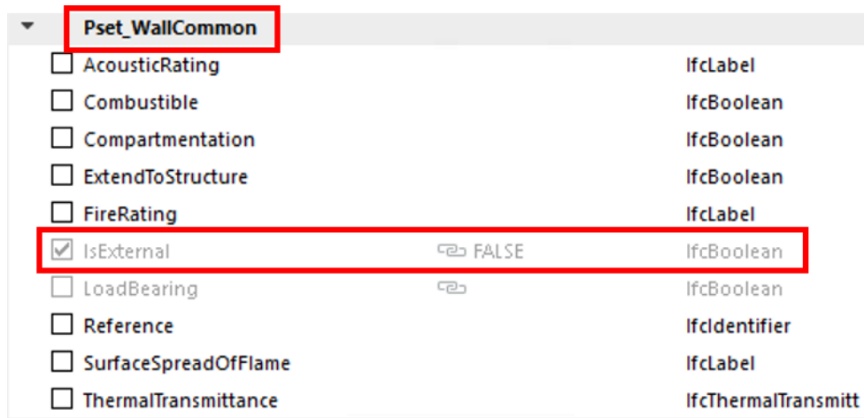
Figure 18 Example of Wall with IsExternal property by modifying selected object setting
