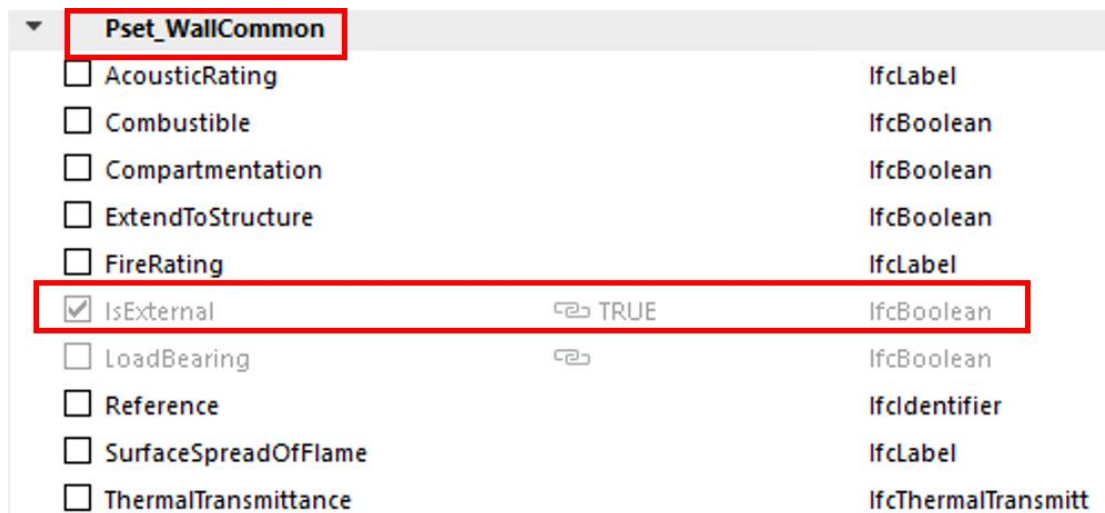
Figure 16 Example of Wall with IsExternal property by changing default setting
